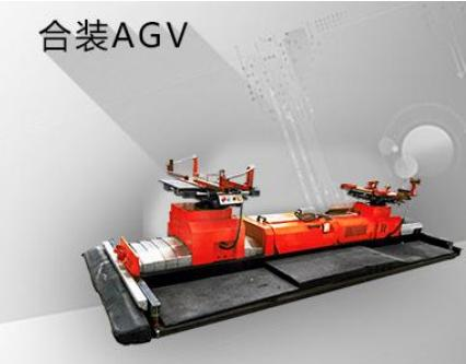
A red and black integrated AGV system featuring two vertical lift arms on a single platform, designed for handling multiple components simultaneously. | 本产品是公司为满足汽车底盘装配线生产环境需求而研发生产的 AGV 产品。可按照车载举升的数量分为单举升合装 AGV、双举升合装 AGV。 | 汽车制造行业          | 磁导航、混合导航 |
